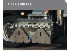
Modular lifting systems with an array of container pick-up options provide fully customized handling of waste containers of 60 to 3,200 l
