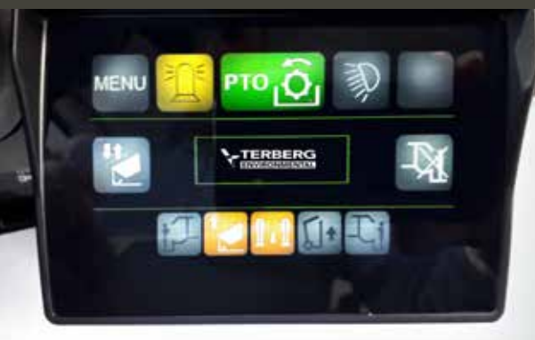
CAN BUS system and management screen in the cab.
