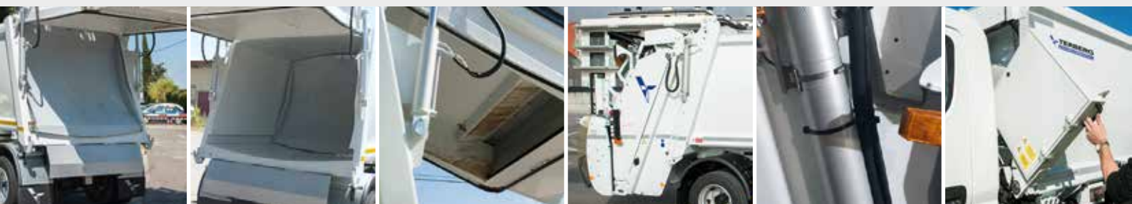
1 Ejector plate perfectly fitted to the body.
