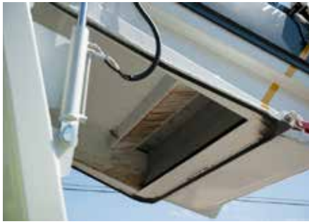
1 Sealing around the entire perimeter of contact between body and tailgate until the maximum height.
