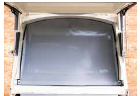
6 Ejector plate perfectly fitted to the body.
