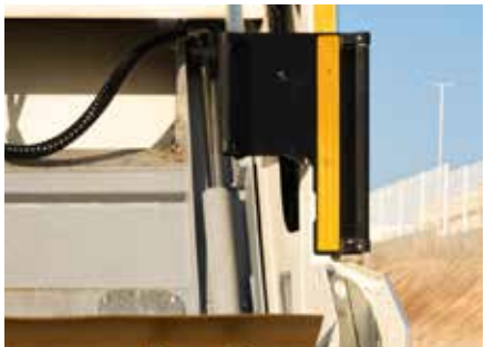
4 External compaction cylinders.
