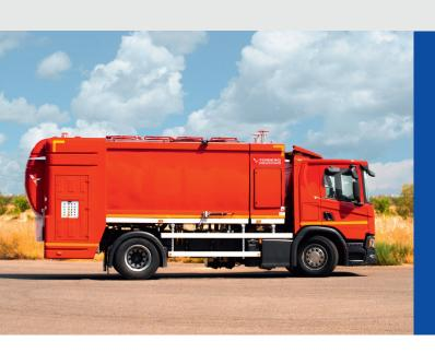
The rear-loading container washing equipment in hot water cleans the bins and containers inside and outside by means of rotating heads and fix bar with nozzles that spray water at high pressure. The container washer is compatible with bins ranging from 80 to 390 liters, flat cover containers with capacities from 500 to 1200 liters and 770 to 1300 liters containers.
