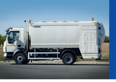
The rear-loading container washing equipment in cold water cleans the bins and containers inside and outside by means of rotating heads and fix bar with nozzles that spray water at high pressure. The container washer is compatible with bins ranging from 80 to 390 liters, flat cover containers with capacities from 500 to 1200 liters and 770 to 1300 liters containers.
