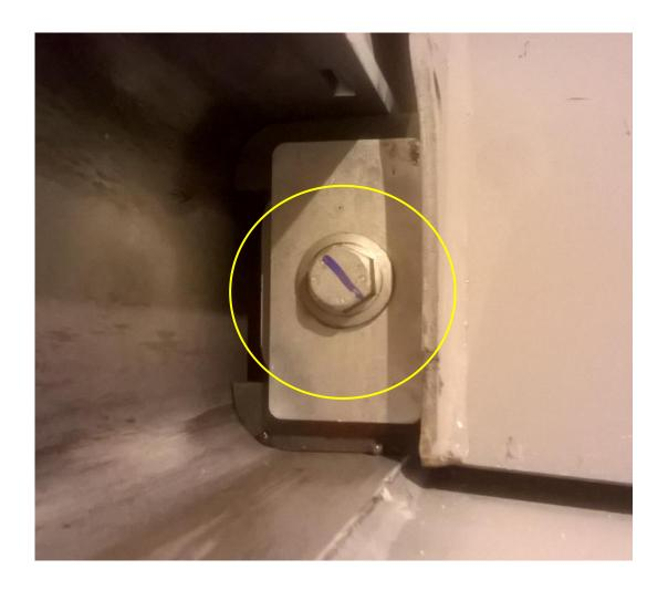
Ensure Barrier Slide Block Retaining Bolt is Torqued to 100Nm and Marked as Per Photograph. Ref Drawing 2000961
