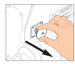
Reset the emergency stop button by pulling it out. The buzzer in the cab stops.
