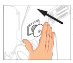
After pressing the emergency stop button, the hydraulic oil supply stops and the electrical circuit is interrupted.
