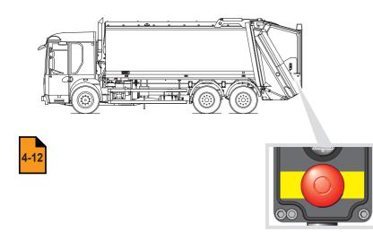
Press yellow push-button to rescue compaction mechanism.
