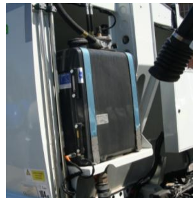
Oil tank at the front of the body
