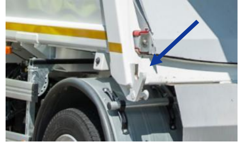
Anchor for automatic lock
