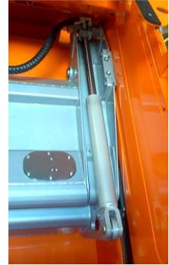
Inverted packer cylinder
