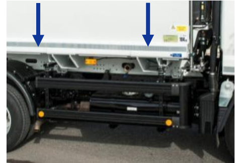
Cyclist protections assembled on the rails
