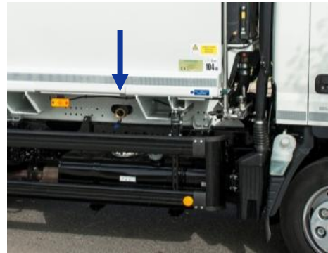
Exterior view of the drain hose
