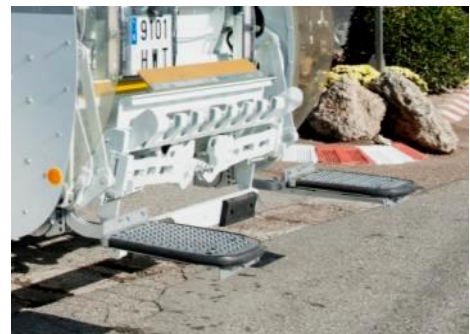
Footboards with weight sensor
