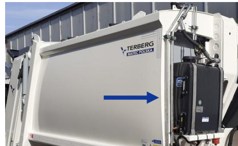
Side view of the oil tank
