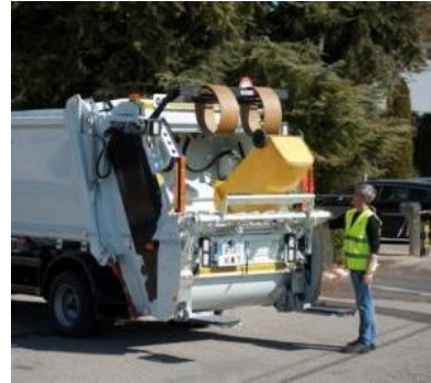
Multi-purpose bin-lifter in up position
