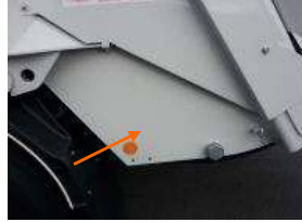
Detailed view with sound absorbing paint and material.
