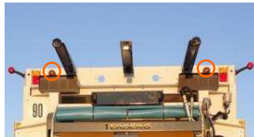
Rear syncro flashing beacons
