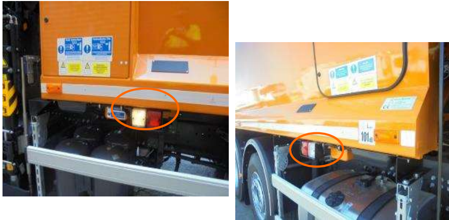
Light for crane indications in both sides of the RCV.
