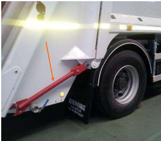
Safety prop in the working position
