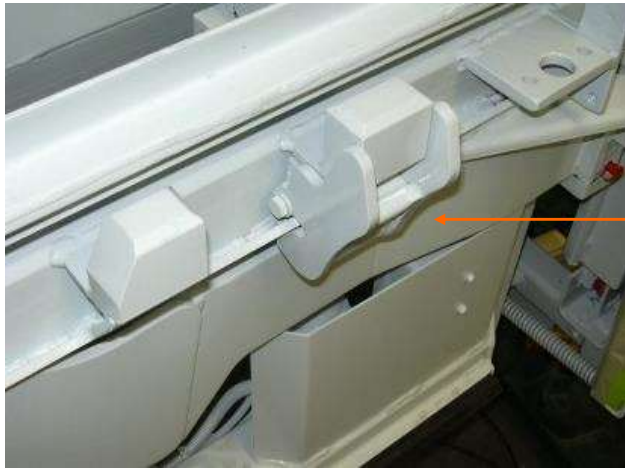
Container presence switch
