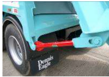
Safety prop in the working position
