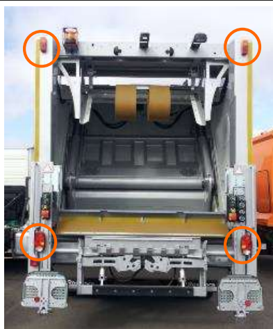
Rear halogen light without protection: standard configuration
