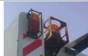
Upper lights with protection
