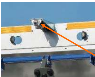
360° view camera (in the same support as standard camera)
