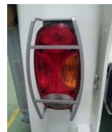
Lower lights with protection
