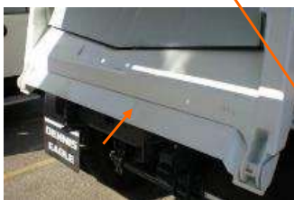
Discharge chute with leachate tank
