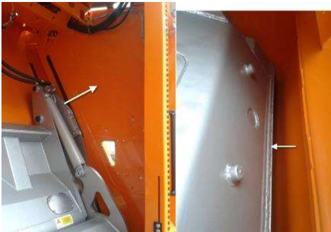
Tailgate sides reinforcement
