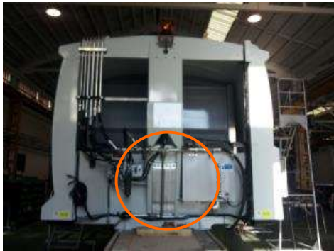
Frontal view of the body with counterweights
