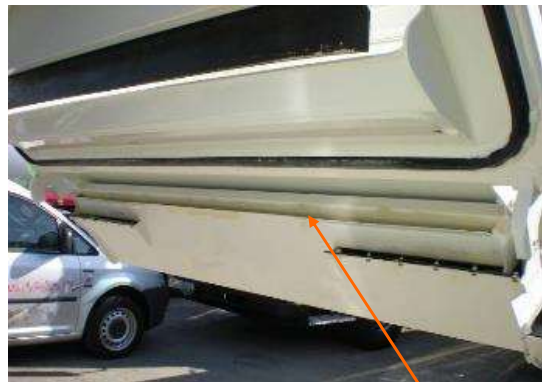
Snap-shut access door system Leachate collector
