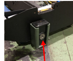
Carriage slide block with wear pads
