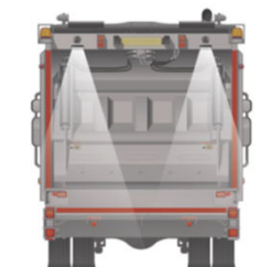
Rear work lights to help crews when working in dark conditions
