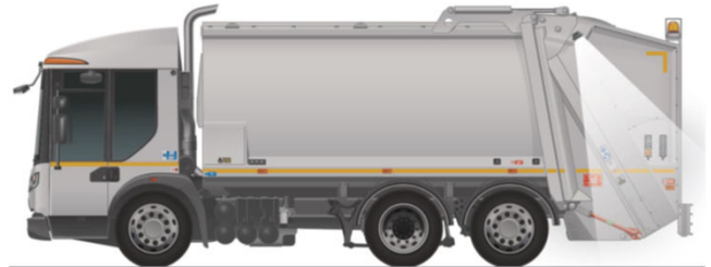
Reverse assist lights shine around the rear sides of the vehicle for a better view when reversing
