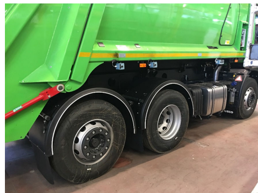
High subframe used here on an Iveco chassis. The customer requested a specific body and chassis combination so the body needed raising to clear the rear axle and reduce the gap between cab and body.
