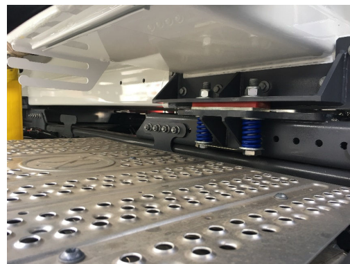
Front subframe section with spring mounting to allow the chassis to flex
