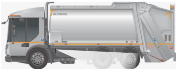
Lower body working lights shine down the side of the vehicle to help with visibility towards the side and rear of the vehicle.
