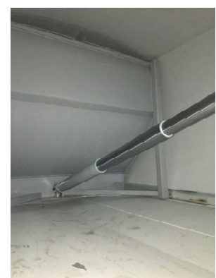
Ejector plate fitted showing hydraulic cylinder extended
