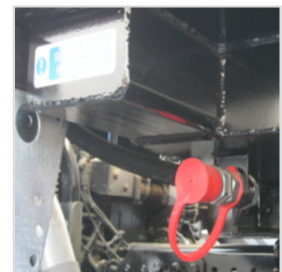
Push fit coupling for the remote filler
