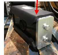
Carriage slide block with wear pads
