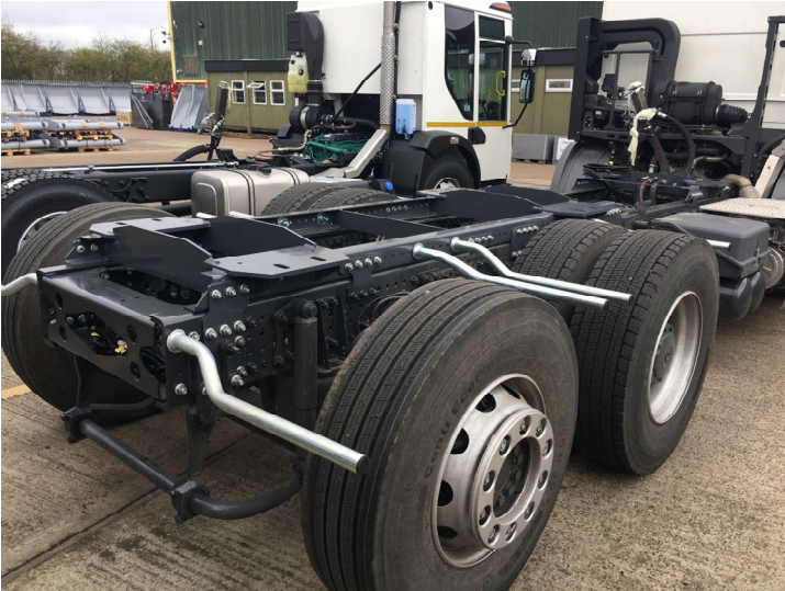
Subframe construction on a Mercedes Econic chassis
