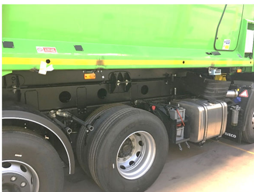
High subframe used here on an Iveco chassis. The customer requested a specific body and chassis combination so the body needed raising to clear the rear axle and reduce the gap between cab and body.
