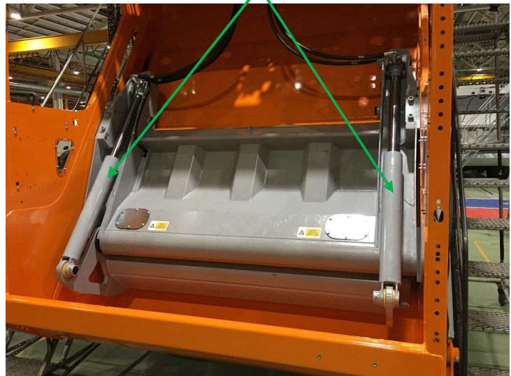
Packer plate hydraulic cylinders
