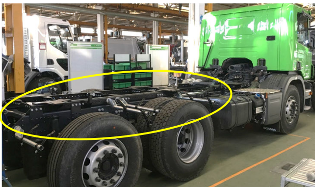
A typical subframe arrangement on a Scania chassis ready to mount the body
