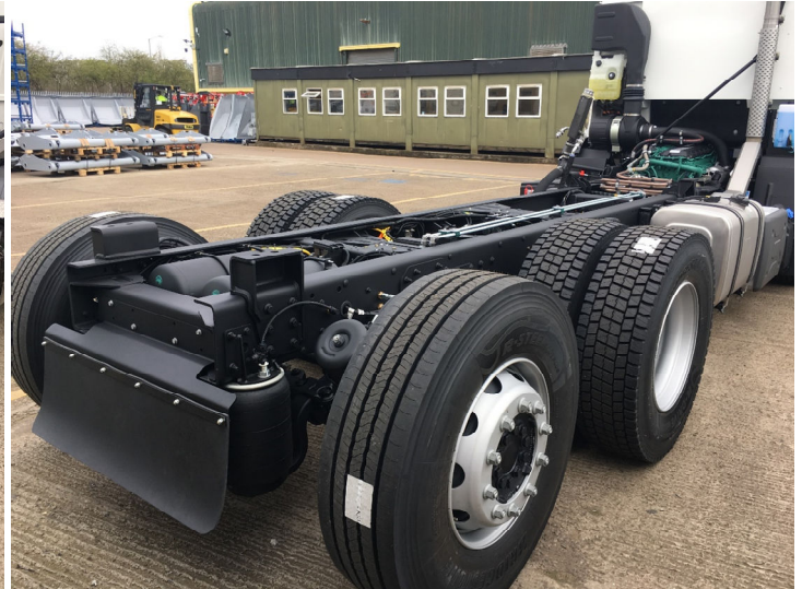
Mounting brackets on an Elite 6 / D Access chassis
