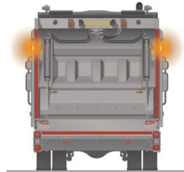
LED beacons at the rear – 2 side
