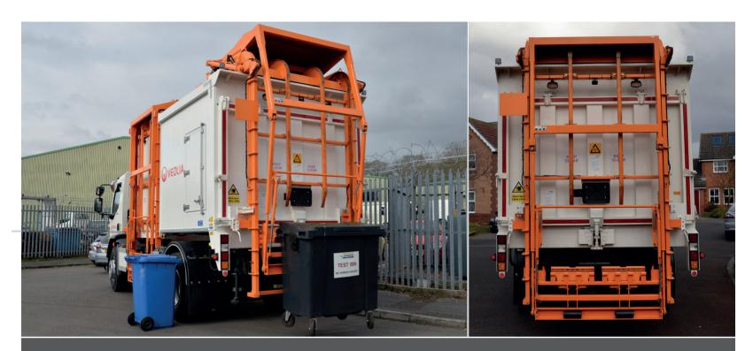
The TLL range of bin lifts provide a practical solution to container collection on existing and new vehicle bodies.
