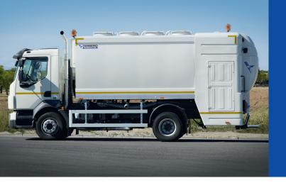
Our superb rear-loading container washer uses cold water efficiently to clean bins and containers. Rotating heads and a fixed nozzle bar deliver high pressure water spray to clean inside and outside. The container washer is compatible with bins ranging from 80 to 390 liters, flat cover containers with capacities from 500 to 1200 liters.
