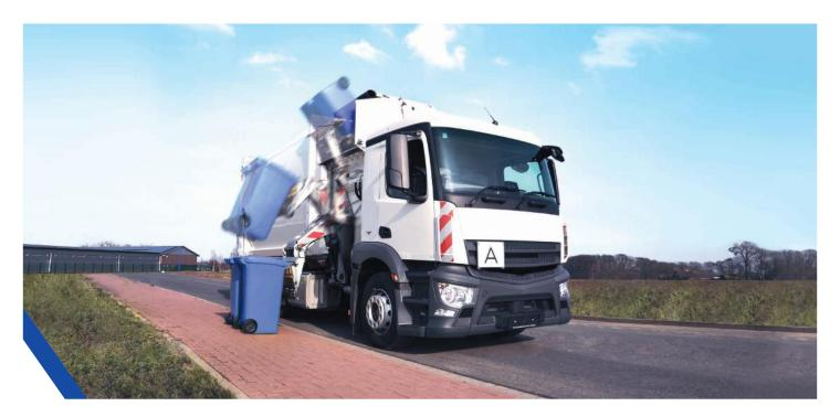
The highest efficiency for any operation: Expand your possibilities with the HS Speedline Scope side loader for the collection of large containers up to 3,200 l.
