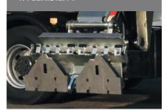
Modular lifting systems with an array of container pick-up options provide fully customized handling of waste containers of 60 to 3,200 I
