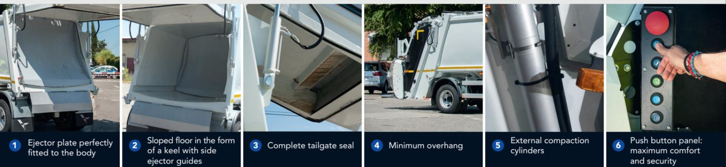
1 Ejector plate perfectly fitted to the body
