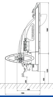
The electrical & hydraulic specifications listed above represent the most common configurations, however, certain chassis/ body combinations may require these to be modified, Terberg engineering should always be consulted before any preparation work commences.
