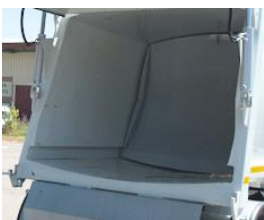
2 Sloped floor with side ejector guides.
