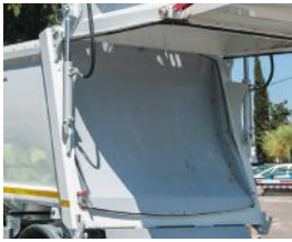
1 Ejector plate perfectly fitted to the body.
