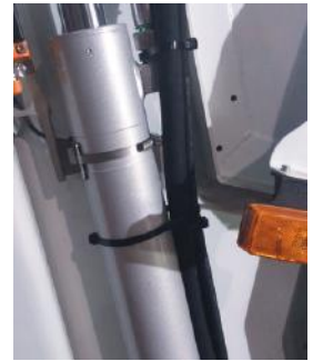
5 External compaction cylinders.
