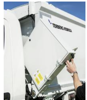
6 Electrical control panel in an easily accessible place.
